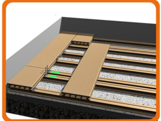
III 、 The end of each decking profile needs to be put on each keel/joist.
