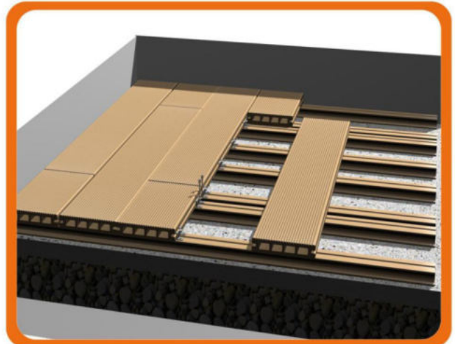
IV 、 Install by buckles/clips one by one
